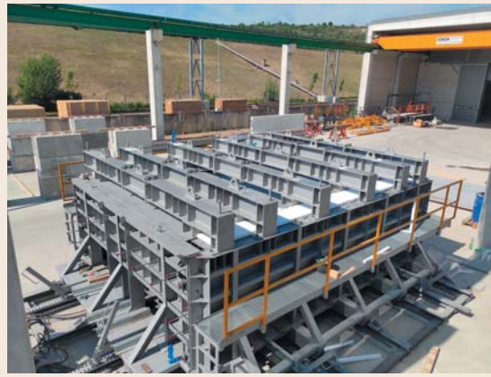
Fig. 8 Cast segment with lifting and turning devices
