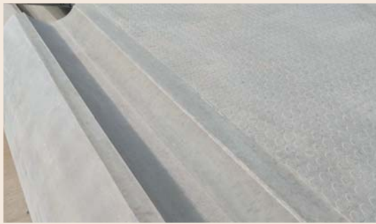
Fig. 5a, b, c UHPFRC segments Fig. 5a, b, c Segmenty z UHPFRC
