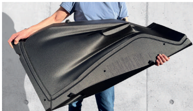
Fig. 12 3D-gedrucktes Schalungselement. 3D-printed formwork element. (© New Digital Craft)
